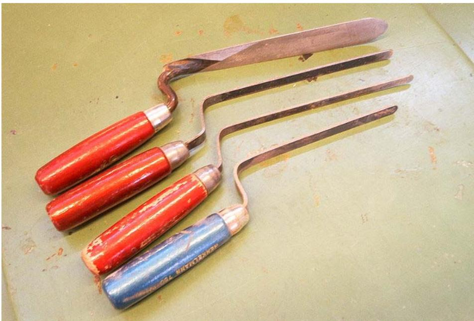
**Figure 1. Examples of jointing tools for finishing joints of different widths.**
