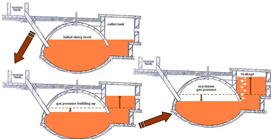
**Figure 2** Initially, the slurry level in the dome and outlet tank are equal (top). When gas pressure starts to build up, the slurry level inside the dome is pushed down, and the slurry is pushed out, so that the level in the outlet chamber rises (lower left). When the slurry level in the dome reaches the level of the exit, gas starts to leak through the outlet chamber. Pressure within the dome is limited by the dimensions at which this leakage occurs.
